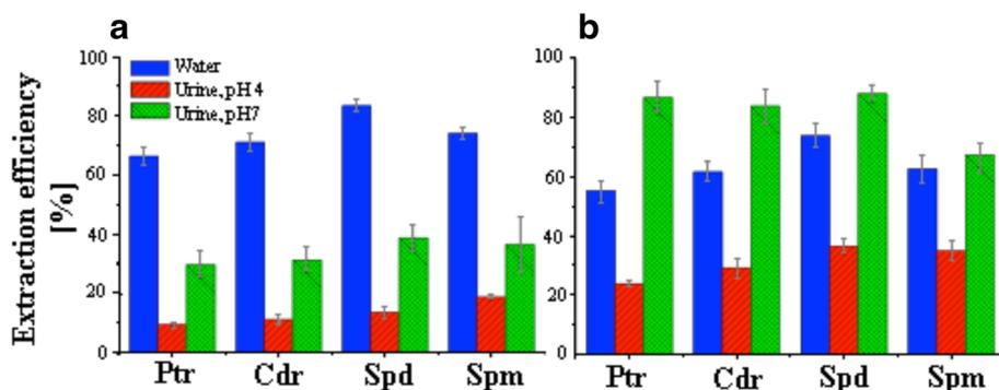
**Fig. 1** Extraction efficiency of putrescine (Ptr), cadaverine (Cdr), spermine (Spm) and spermidine (Spd) from urine by flat sheet supported liquid membrane in dependence of pH of the acceptor phase: (a) 0.1 M HCl as acceptor phase, (b) 1 M HCl as acceptor phase. Concentration of polyamines in donor phase is 50  $\mu$ M
