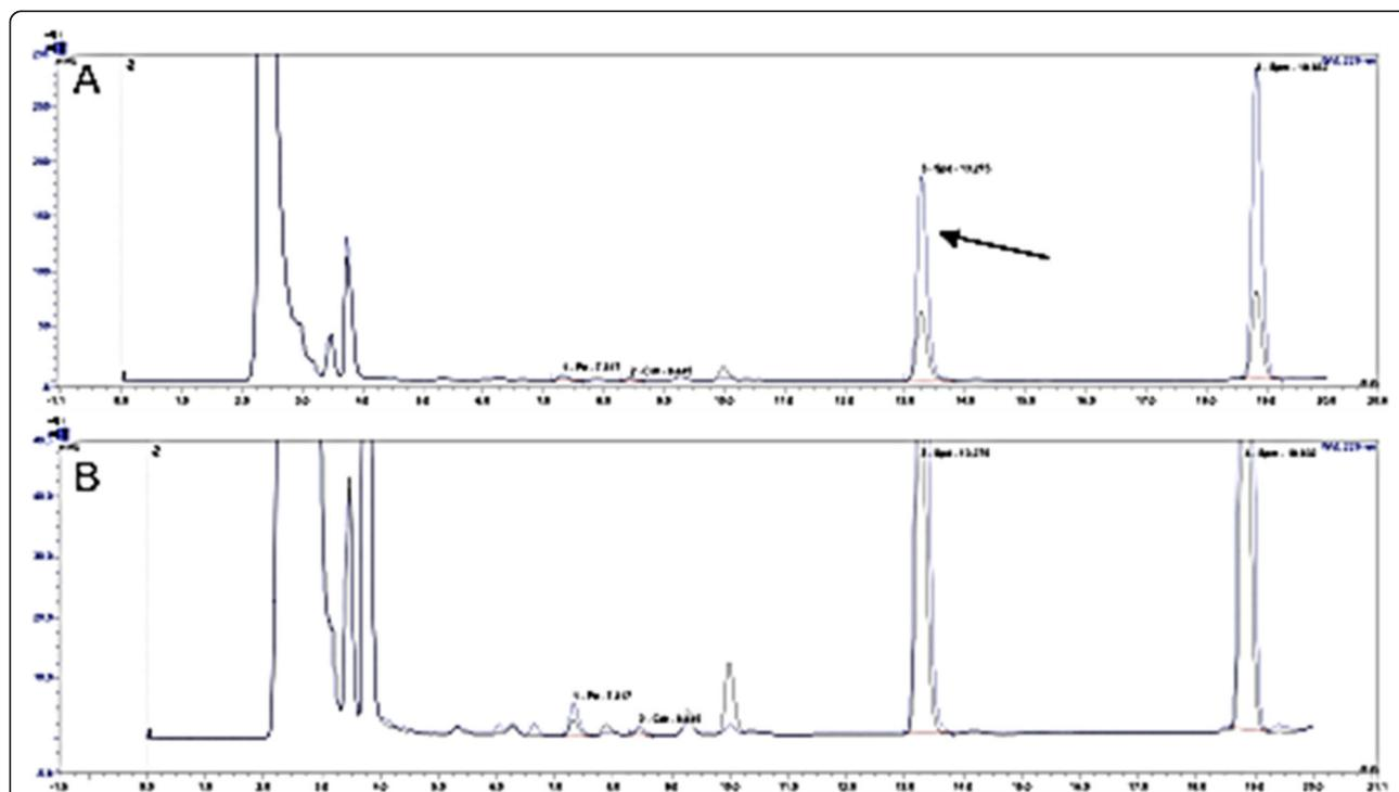
**Fig. 3** Unspiked porcine kidney homogenate (a) and its supported liquid membrane extract polyamines (b) studied by HPLC. Extraction conditions: 0.5 M HCl as an acceptor phase and extraction time - 45 min
