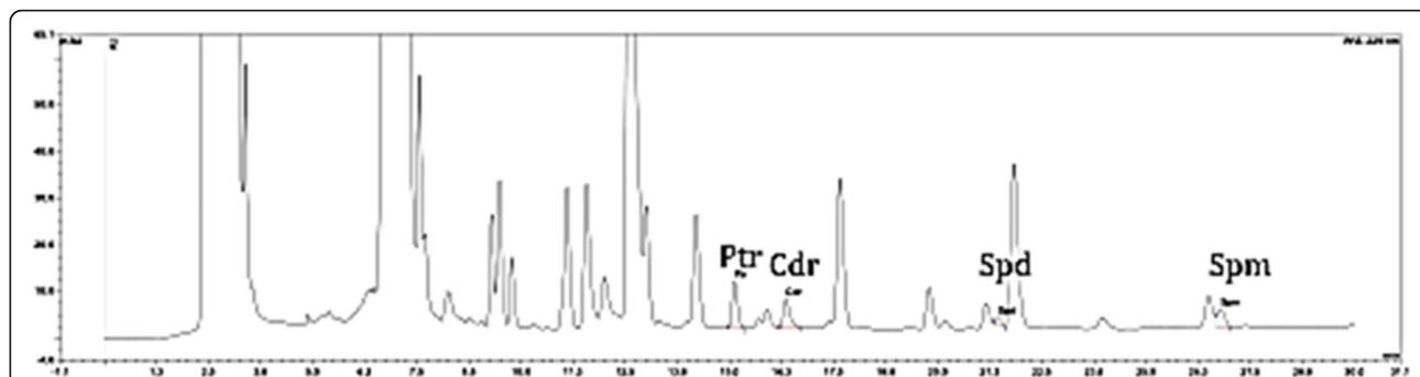
**Fig. 2** Single hollow fiber supported liquid membrane extract of polyamines from unspiked urine of healthy person. Symbols of amines are as in Fig. 1. The elution program was convex gradient from 20% acetonitrile in water to 80% in 30 min
